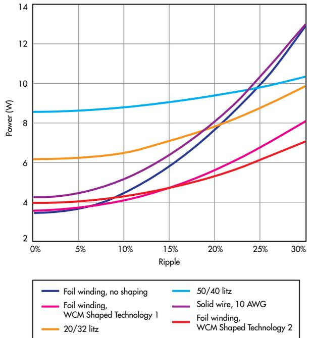
8. At 100 kHz, power losses through the windings jump significantly over those at an operating frequency of 10 kHz.
