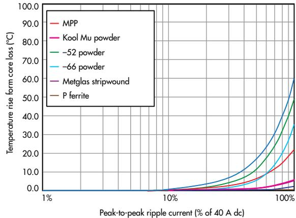
5. Factoring temperature rise and peak-to-peak ripple current into the mix, common core materials perform well at 10 kHz.
